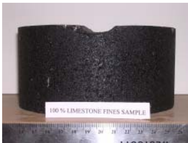
Figure 4.30 Typical rut depth for 100 percent limestone sample
