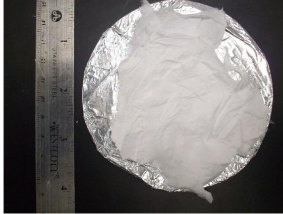
Figure 4.4 Picture of a 4 inch diameter sample collector after electrospinning experiment, the white sheet is the YSZ raw fiber mat
