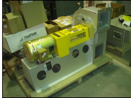
Figure 19: Cincinnati Blower model RBE-9 used to pull dilution air/exhaust mixture through the dilution tunnel.
