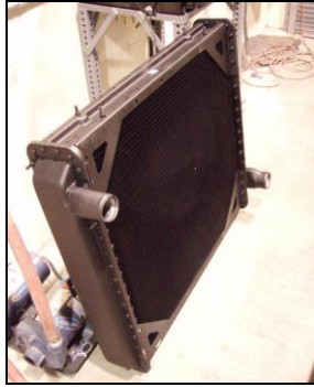
Figure 16: Freightliner radiator to be used for rejecting heat generated within the main water tank during testing.
