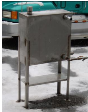
Figure 10: Stainless steel system water supply tank.
