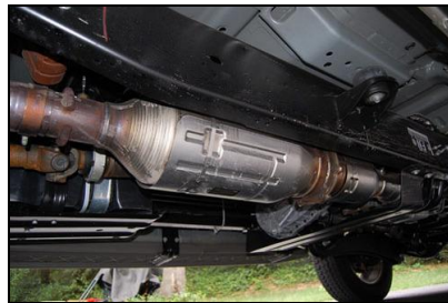
Figure 9: Diesel Particulate Filter, as installed in the exhaust system of a Ford F-250 Super Duty Diesel truck [42].
