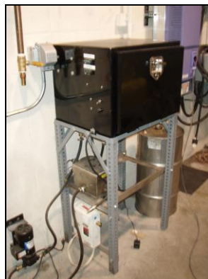
Figure 18: Fuel conditioning and weighing box for small engine test cell.
