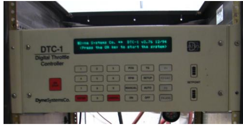
Figure 23: DTC-1 used for SETC fuel rack control.
