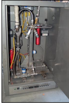
Figure 36: CFR 1065 compliant 1065 sampling system.
