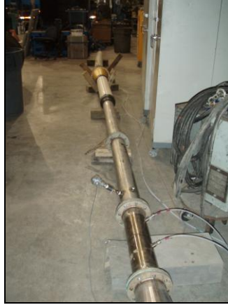
Figure 33: Venturi flow meter calibration setup.
