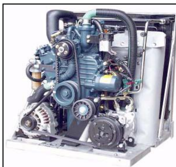
Figure 2: Photograph of typical APU system [8].
