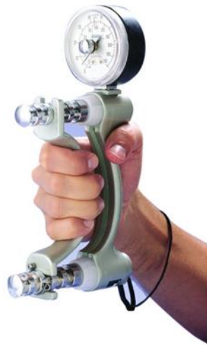
Figure 2: Power hand grip using Jamar hand dynamometer.
