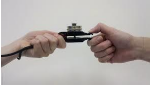
Figure 1: Key pinch grip using a Jamar pinch grip sensor.
