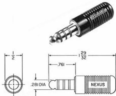
Figure 88 - Nexus TP-101 (U-174/U) Plug
