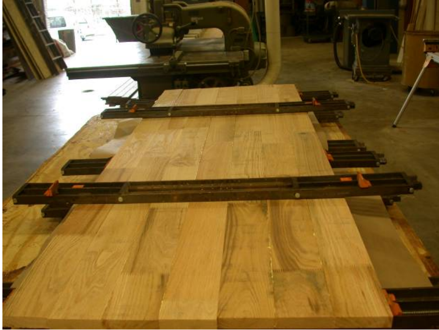
Figure 3.9 Production of edge-glued panels using panel clamps.
