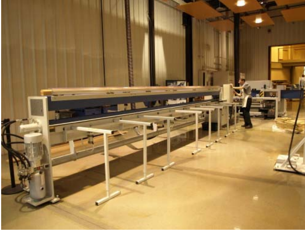
Figure 3.7 Grecon Profijoint machinery and press used to produce vertical finger-joints.
