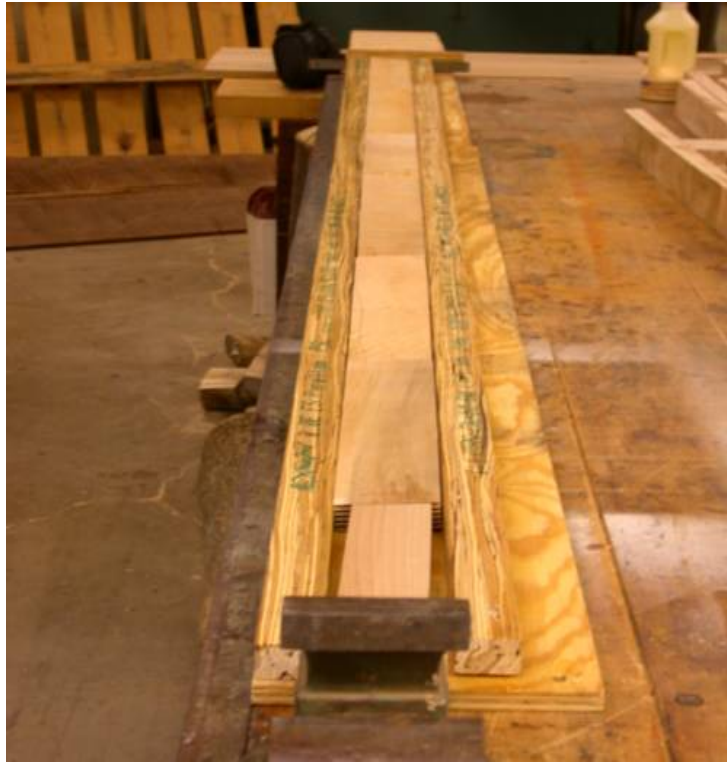
Figure 3.6 Press used for manufacturing finger-jointed lumber at DOF.
