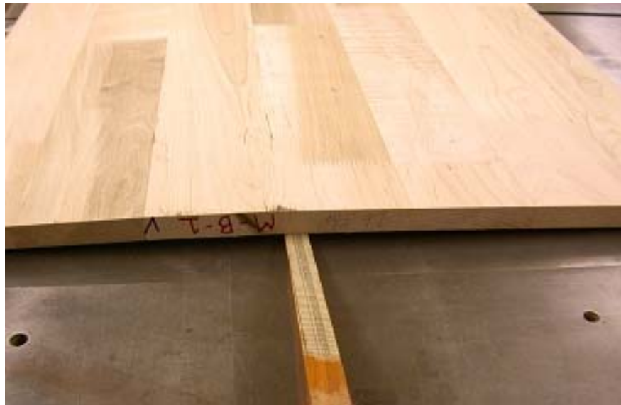
Figure 3.10 Measurement of warp (cup) using a calibrated wedge.
