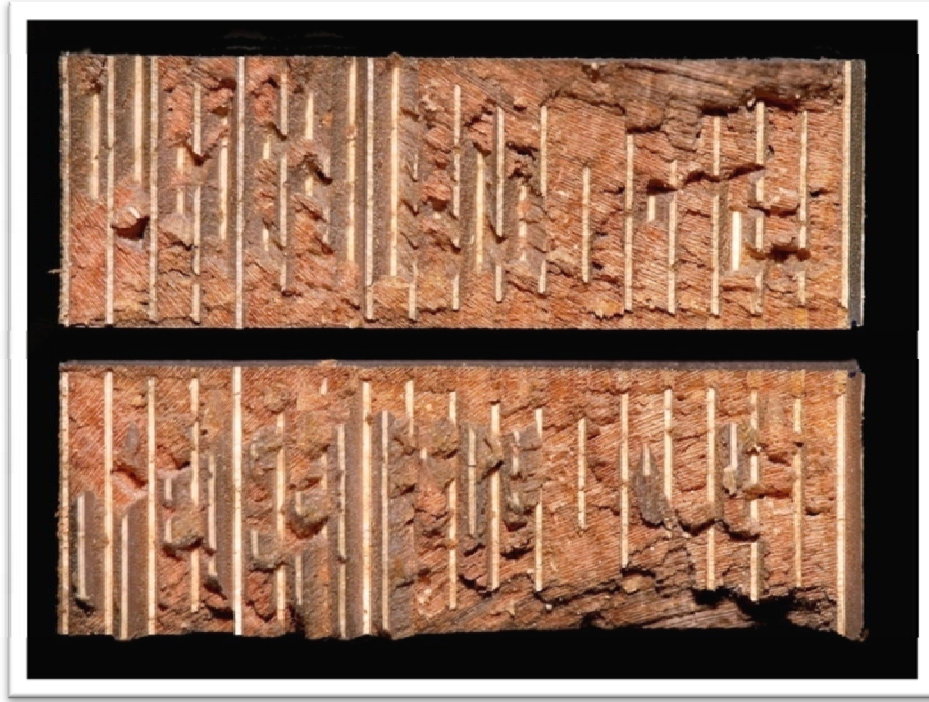
Figure 4.8 90% wood-failure of vertically finger-jointed cherry test specimen.
