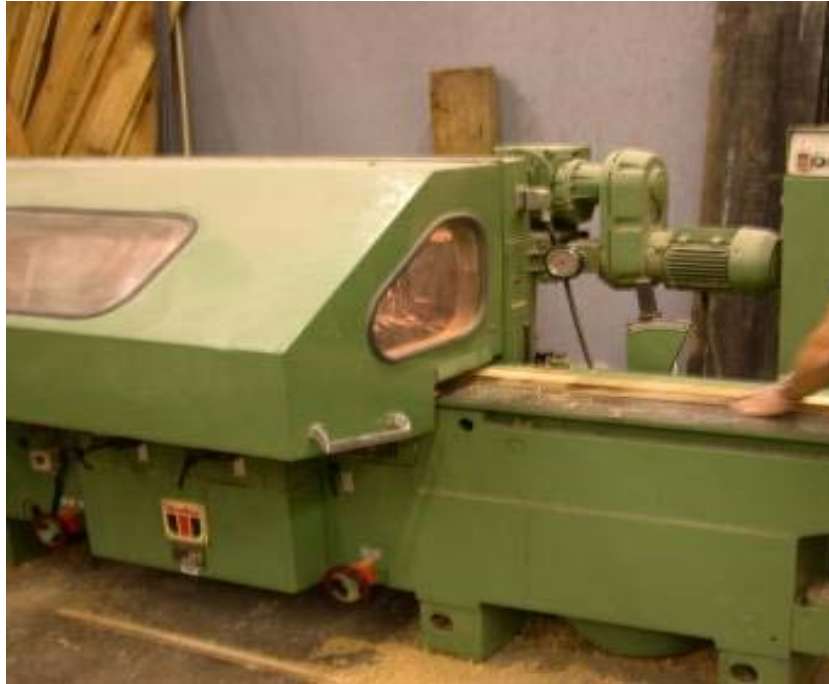
Figure 3.8 Four-head moulder used to prepare blanks for edge-gluing.
