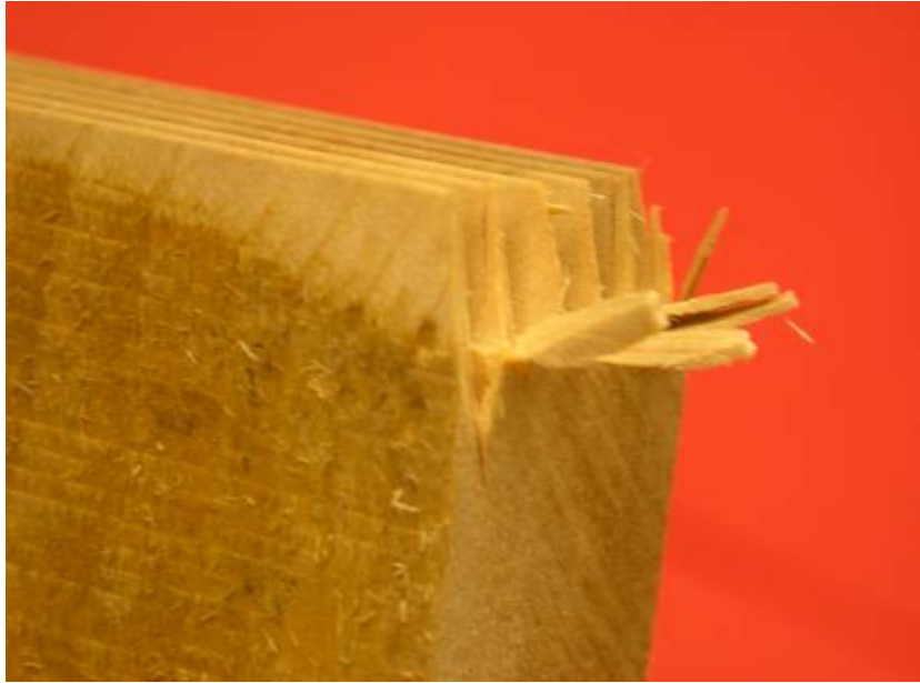
Figure 3.4 Tearout in horizontal finger-joint caused by high feed-rate.
