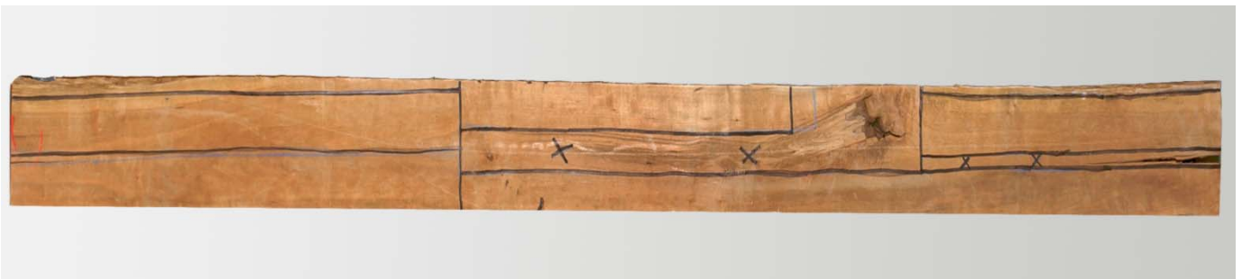
Figure 3.1 Example of cutting pattern used to salvage rough lumber.
