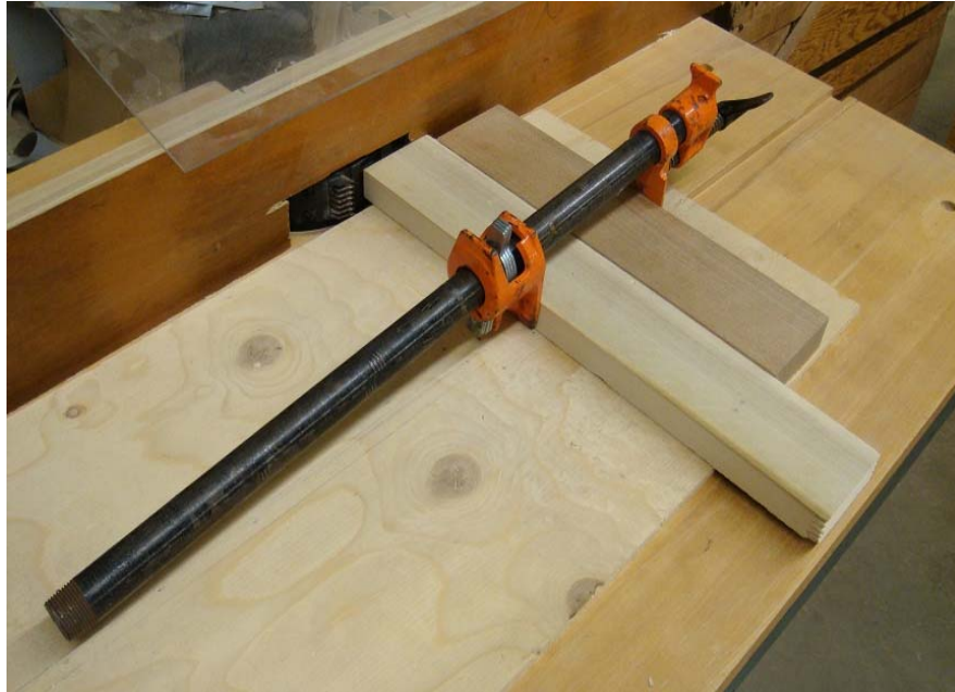
Figure 3.3 Shaper set-up used for manufacturing horizontal finger-joints.
