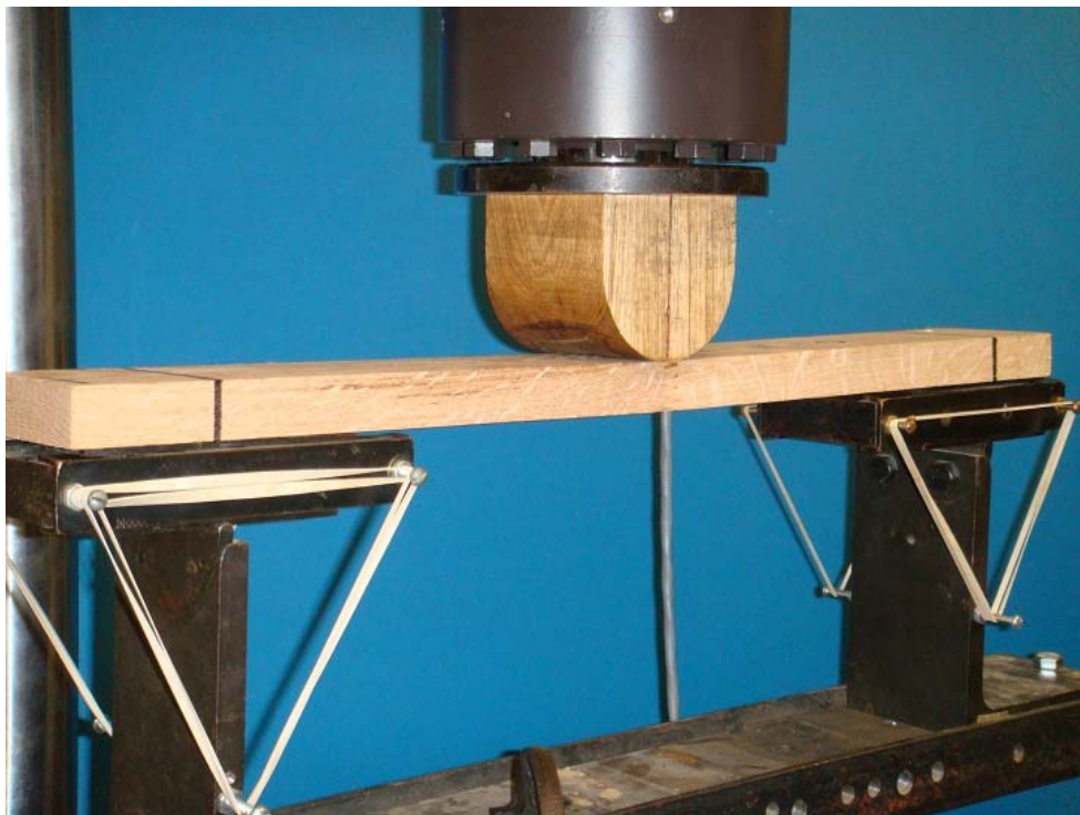
Figure 3.12 Determination of MOE and MOR of horizontally finger-jointed red oak test specimen by static three-point bending.
