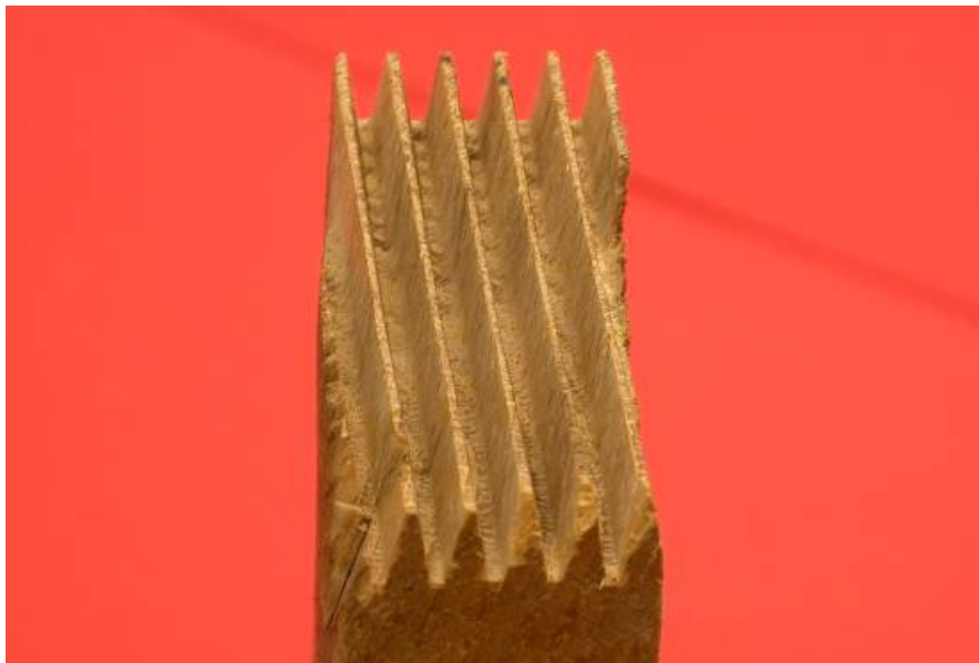
Figure 3.5 Specimen with slanted fingers produced from warped shorts.
