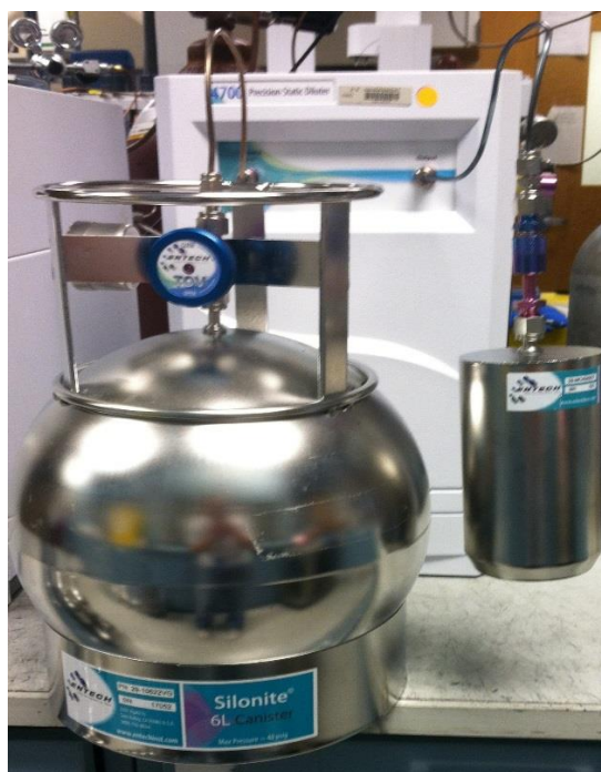
Figure 3. Entech 4700 6-L to 450 cc Canister Transfer
