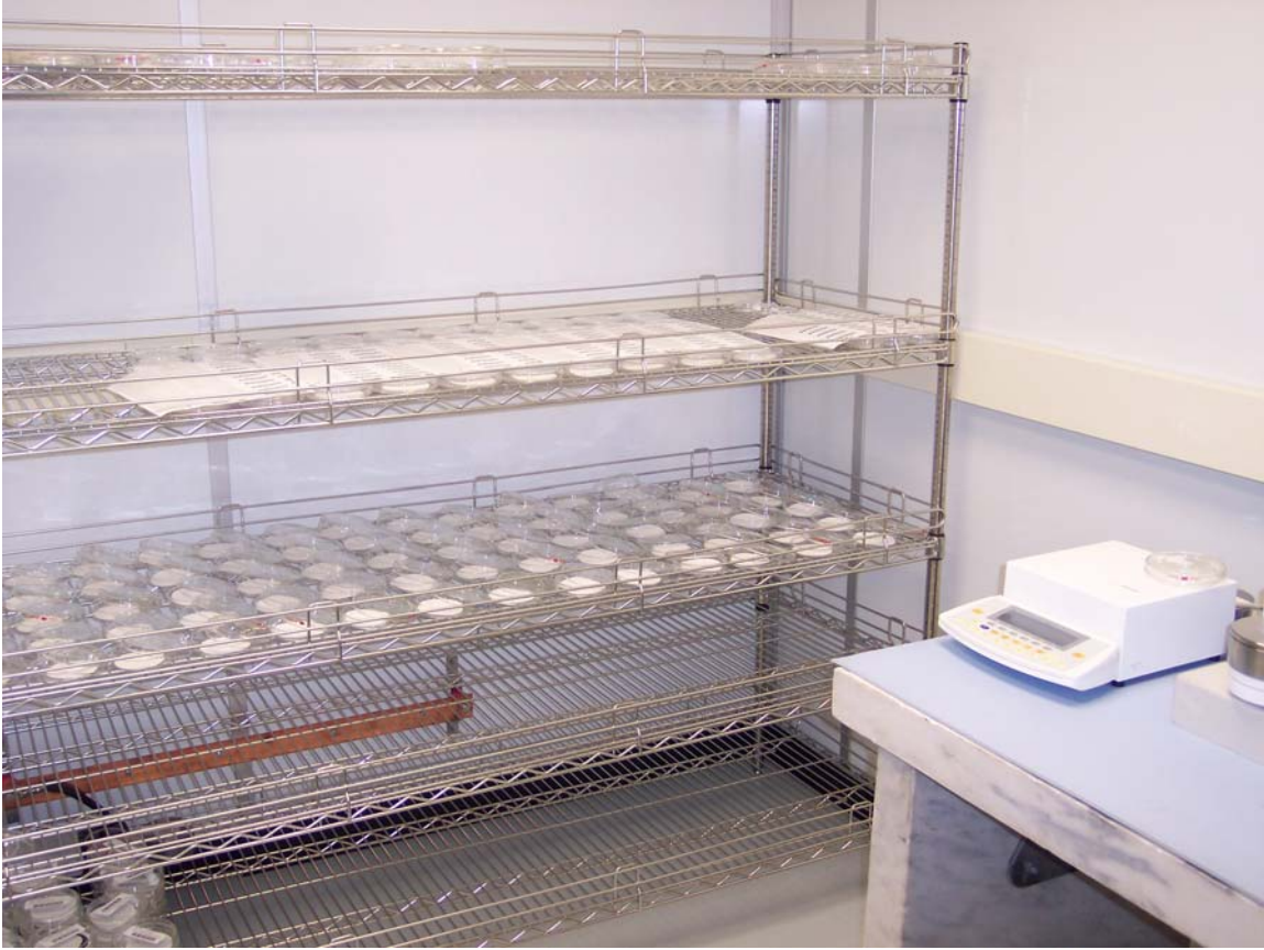
Figure 3-3: Shelves containing pre-weighed filters and conditioning filters
