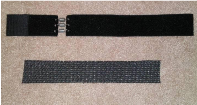
Figure 6. Velcro® band (with springs) and foam barrier from top to bottom, respectively.
