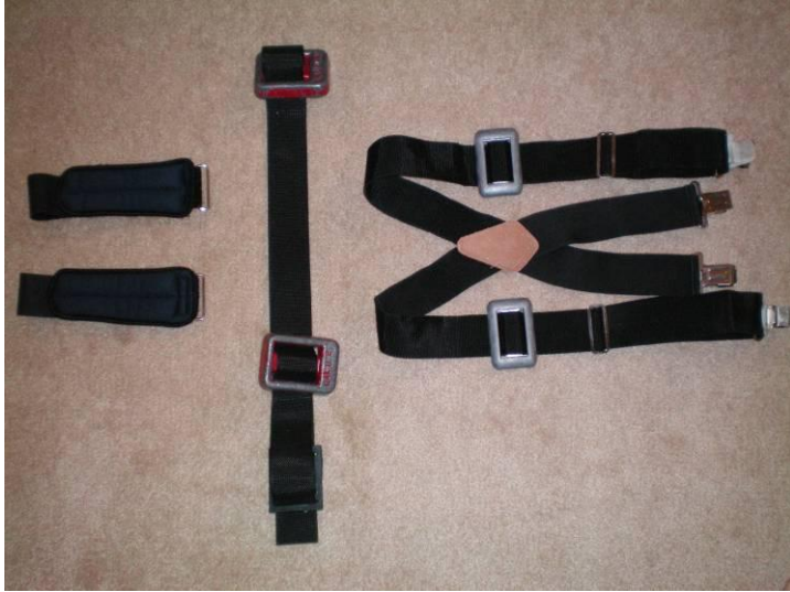
Figure 7. Mass used on wrists, lower torso, and upper torso (from left to right).
