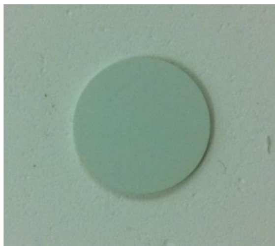
Figure 77: Bisqued anode support at 1100^{\circ}\text{C} .
