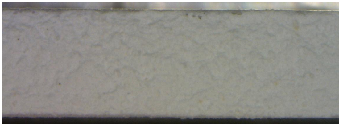
Figure 75: Anode support cross-section demonstrating good lamination.
