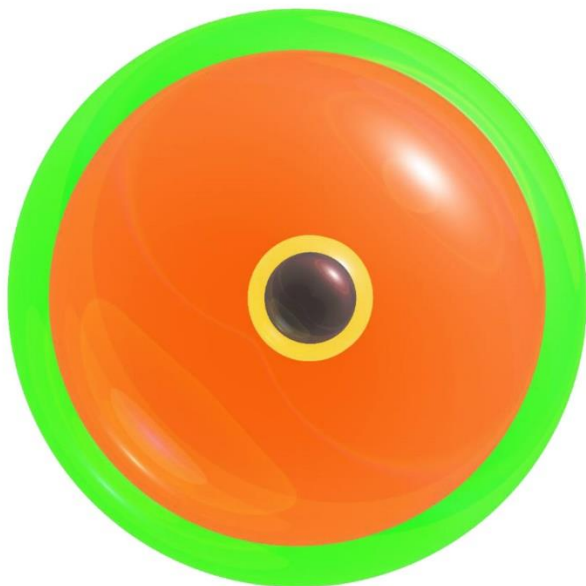
Figure 2.6. To-scale diagram of contribution of various SPION layers to hydrodynamic diameter (determined by DLS).
