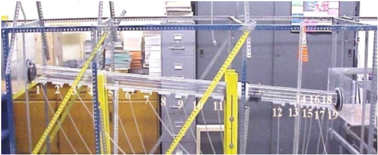
Figure 3.10 Piezometer tap locations
