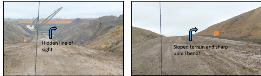
Figure 4.1: (On left) mud pile causing hidden line of sight. (On right) sloped terrain.
