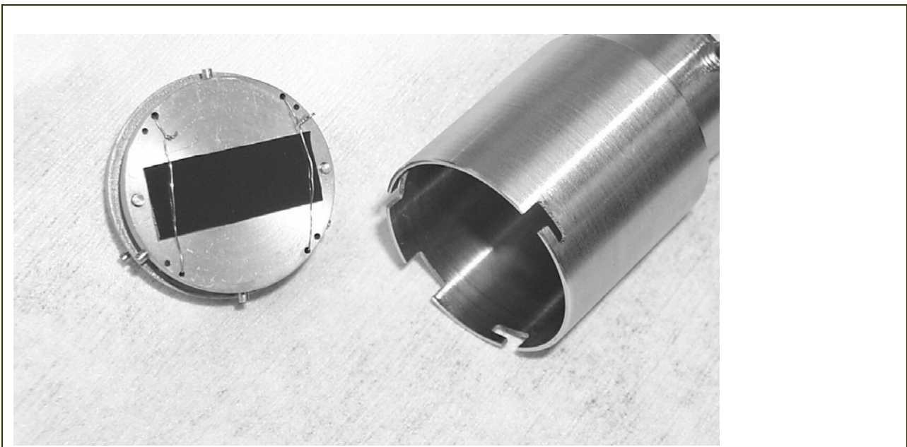
Figure 3-2. Sample holder with sample and notched end of receiver. (Courtesy: K. Ziemer)
