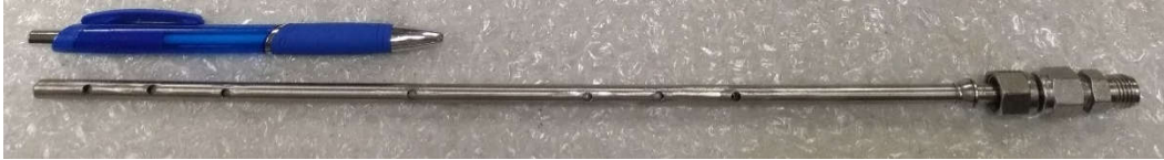
Figure 23 The final pitot tube for flow rate measurement.
