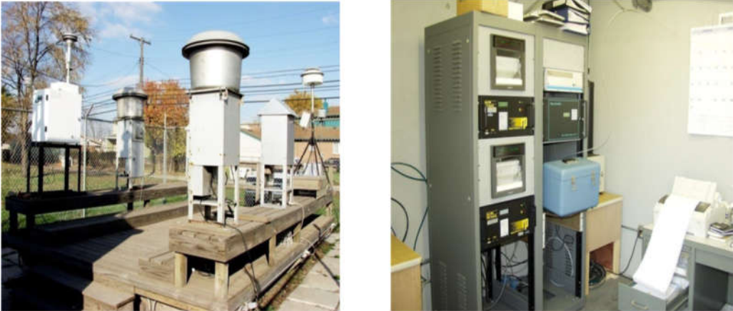
Figure 1 Typical US EPA stations for monitoring ambient air near highways and selected locations [8].
