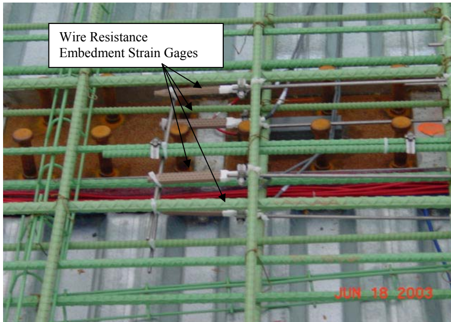
Figure 3.4: Wire Resistance Embedment Strain Gages (photo courtesy of Dr. Shoukry, WVU)
