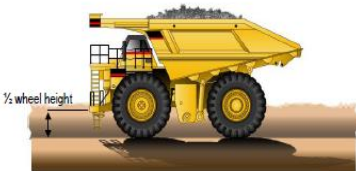
Figure 4.28 Minimum safety berm height (Holman, 2006)
