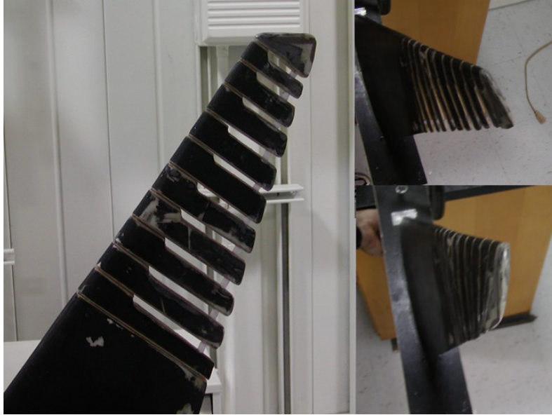
Figure 60– Spring 2006 modifications to the adaptive washout mechanism which include rounding of trailing edges, new Nylon restraining monofilament and Teflon spacers between trailing edges of each free floating wing section.
