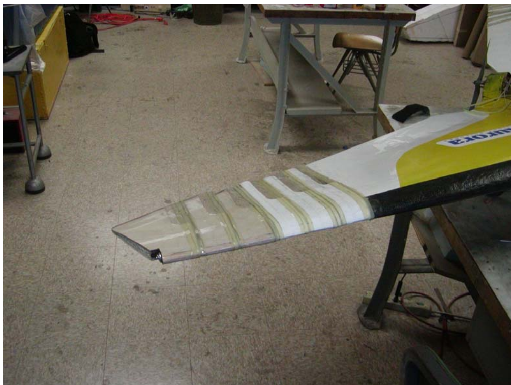
Figure 133 – Completed morphing wing section covered by polypropylene and laytex skin.
