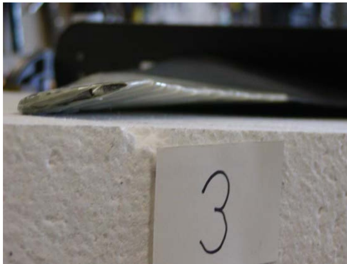
Figure 52– Control position 3 in the morphing wing which corresponds to a +7 degree twist of the tip.
