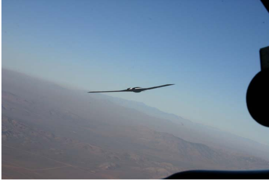
Figure 30 – Lockheed Polecat high altitude UAV which will in the future use wing morphing for control. ( http://www.lockheedmartin.com/wms/findPage.dsp=fec&ci=17787&rsbci=0&fti=1 )
