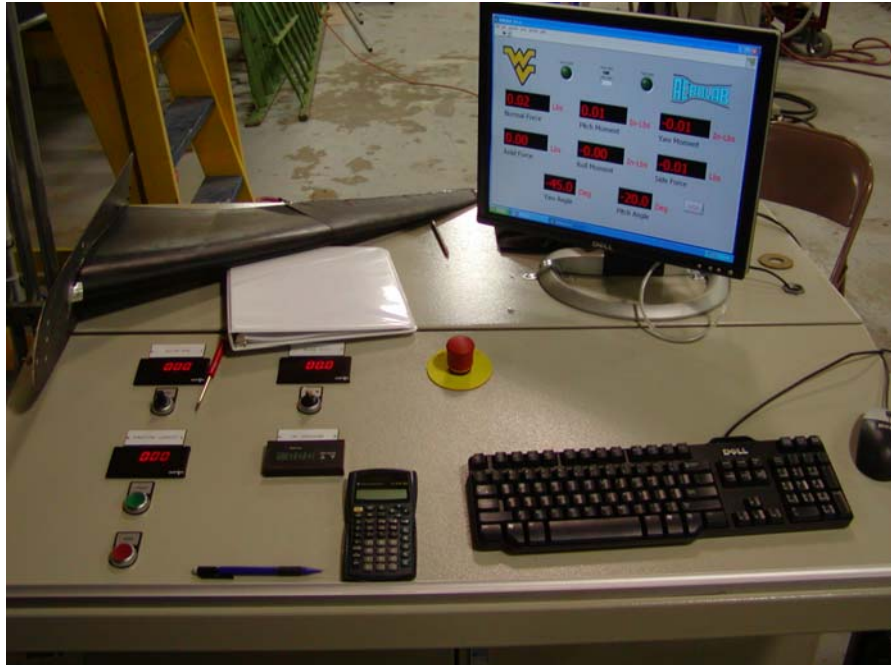
Figure 66– Data acquisition computer interface mounted on a new shielded and grounded enclosure.
