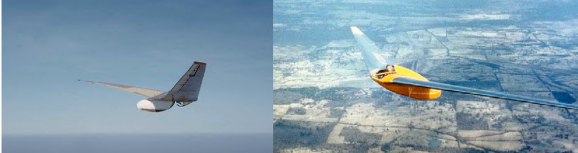
Figure 18 - The Horten IV during flight testing at Mississippi State University. The unaltered Ho IV with original landing skid can be seen on the left and the right shows the fairing built during testing in an attempt to improve the aircraft's performance. (Bullard, 2003)
