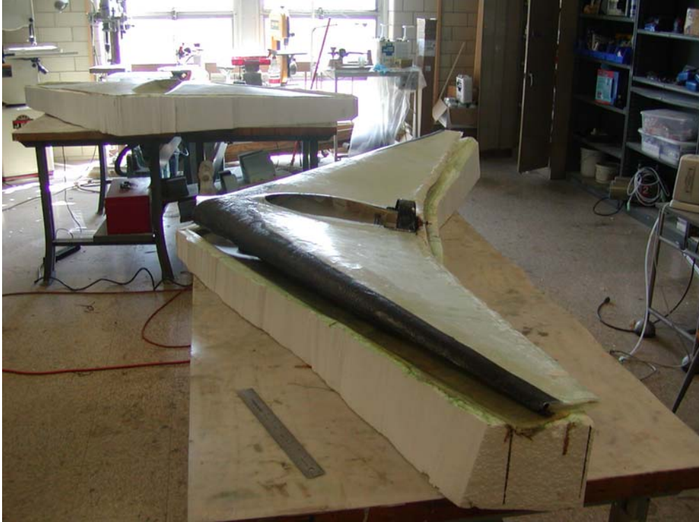
Figure 129 - Female molds with the upper skin bonded to the carbon cuff.
