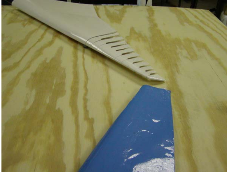
Figure 48 – WVU 1st Generation 610 mm span wind tunnel model in blue, showing obvious skin buckling.
