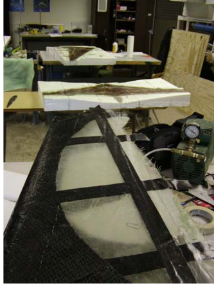
Figure 47 – First generation composite skin made of woven glass and carbon and unidirectional carbon.
