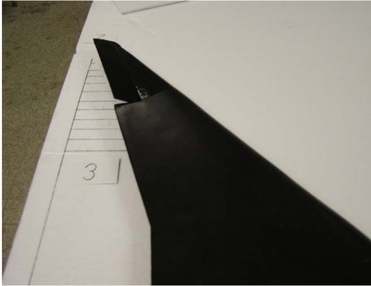
Figure 53– Control position 3 as seen on the elevon equipped comparison wind tunnel model.
