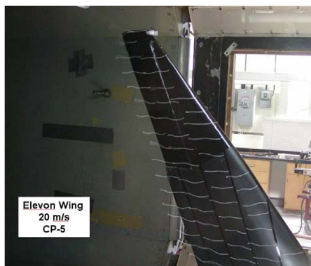
Figure 87- Elevon Wing at 68 ft/sec (21 m/s), 7 degree AOA and with a -3.5 degree control deflection.
