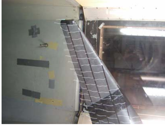
Figure 149 - Morphing Wing at 20 m/s, 7 degree AOA and control position of approximately -2 degrees. Note the apparent lack of tip vortex.
