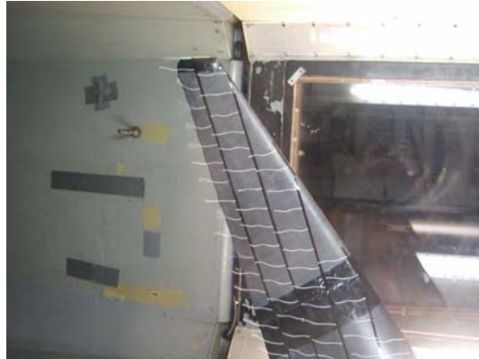
Figure 89- Morphing Wing at 68 ft/sec (21 m/s), 7 degree AOA and with an approximate -2 degree control deflection. Note lack of tip vortex
