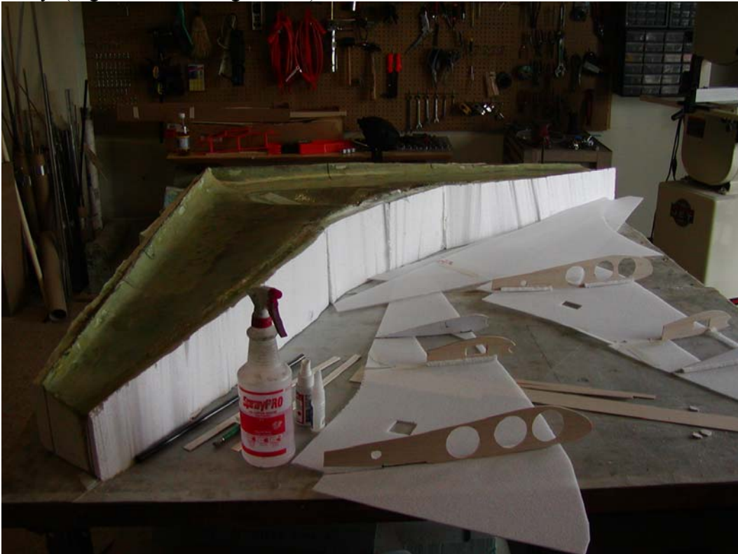
Figure 128 - Full scale lower skin mold with Rohacell cores and glass/balsa ribs in foreground.
