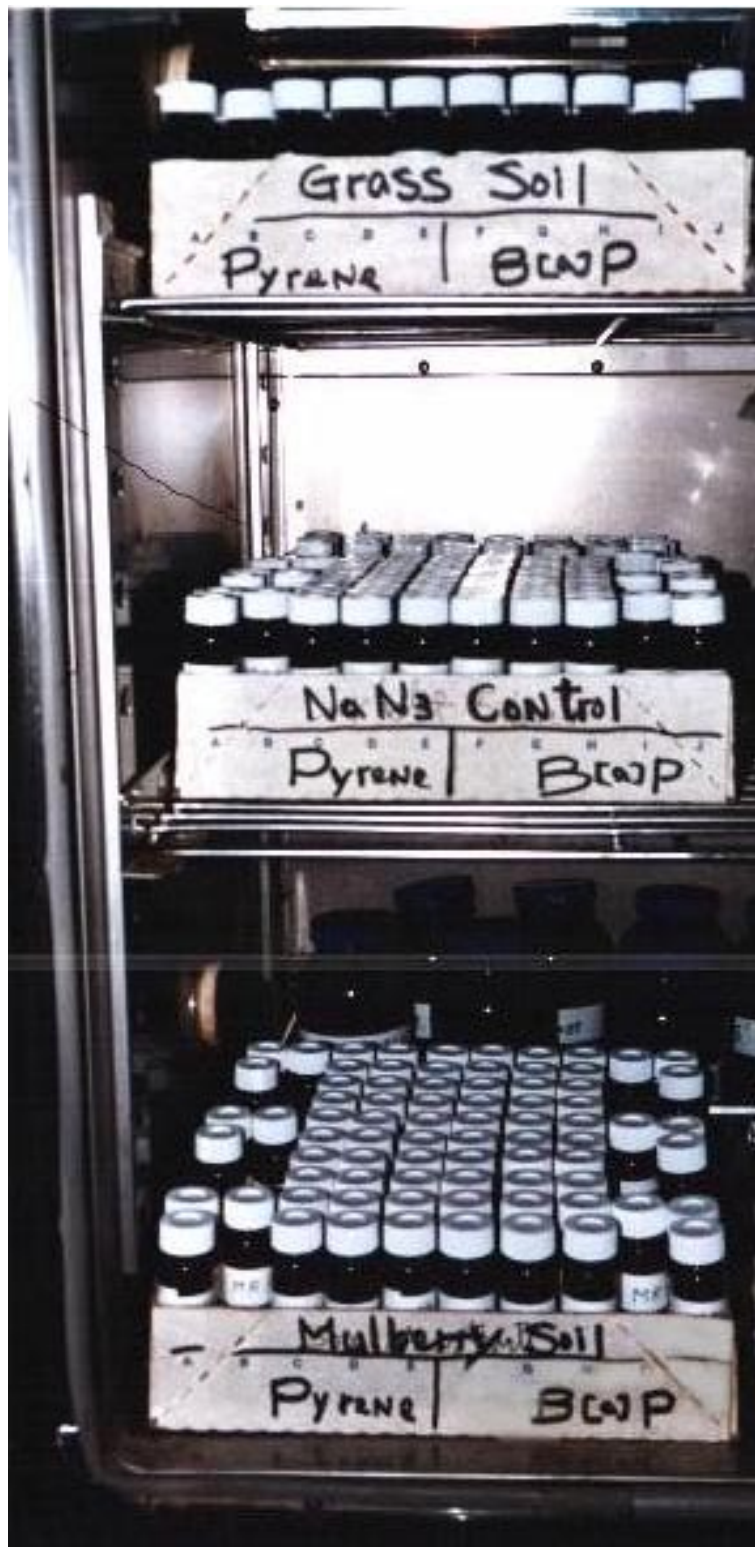
Figure 3.5. Soil microcosms setup in the environmental chamber
