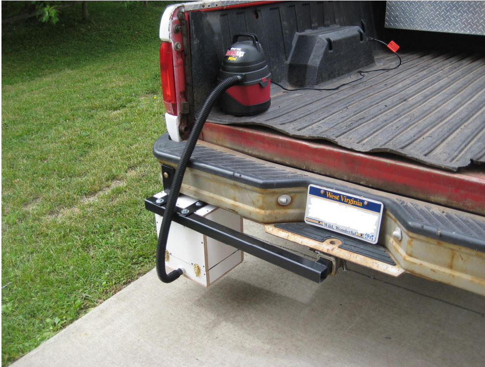
Figure 5.2 Rear View of Dust Collector Mounted to Bumper of Test Vehicle
