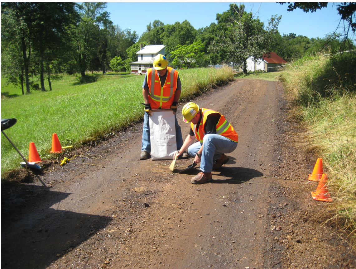
Figure 5.5 Collection of a Surface/Bulk Dust Loading Sample
