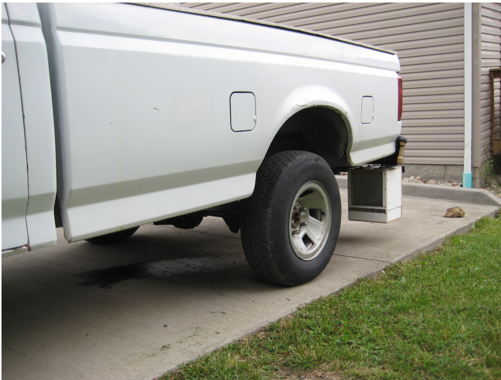
Figure 5.3 Opening of Filter Box Facing the Rear Wheel of Test Vehicle
