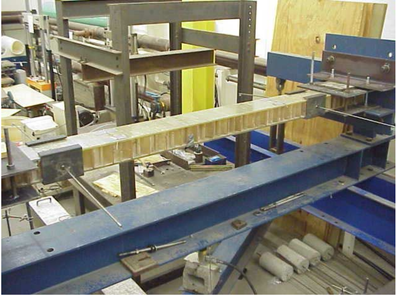
Figure 5.8 End-Clamps for Torsion Testing of Transverse Samples
