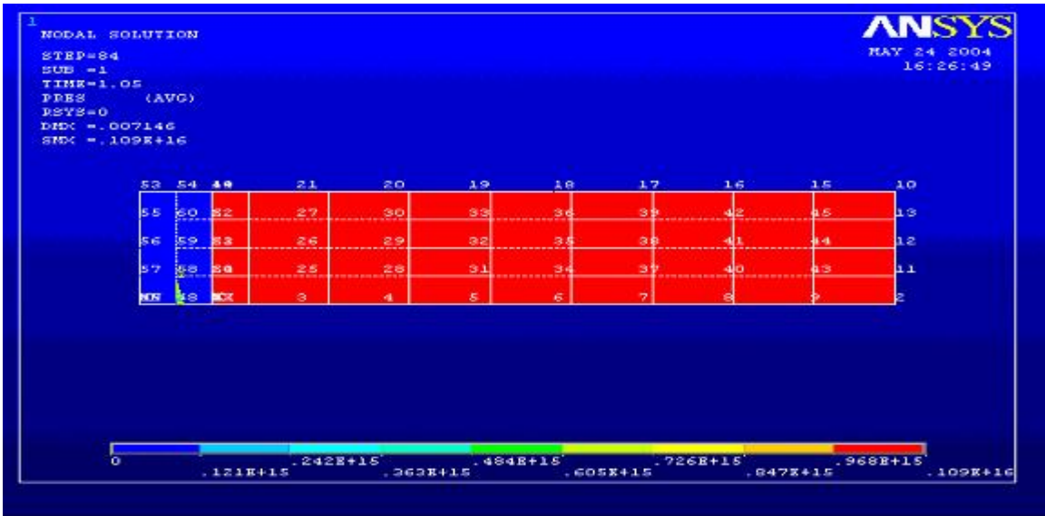
Figure 16 Pressure plot for fluid element when amplitude is 0.85 mm and angular velocity is 3.0 sec -1
