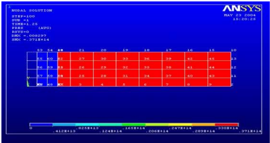
Figure 11 Pressure plot for the fluid element when amplitude is 0.5 mm and angular velocity is 2.5 \text{ sec}^{-1}
