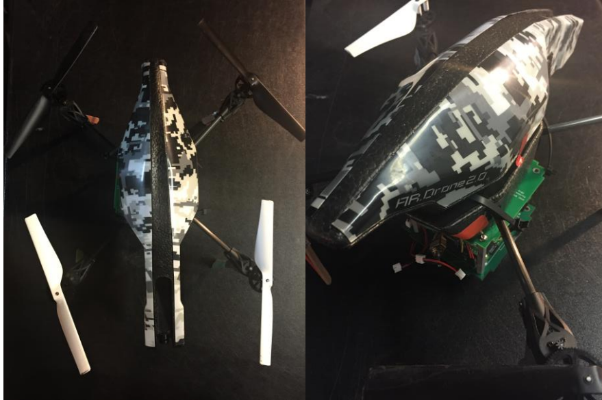
Figure 57: NDVI Payload Attached to the Parrot AR.Drone Quadcopter
