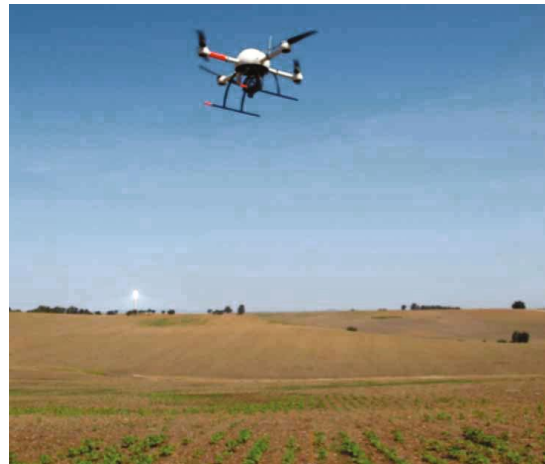
Figure 6: Flight Testing of Quadcopter UAV (Model MD4-1000) over Experimental Sunflower Crop-Field [21]
