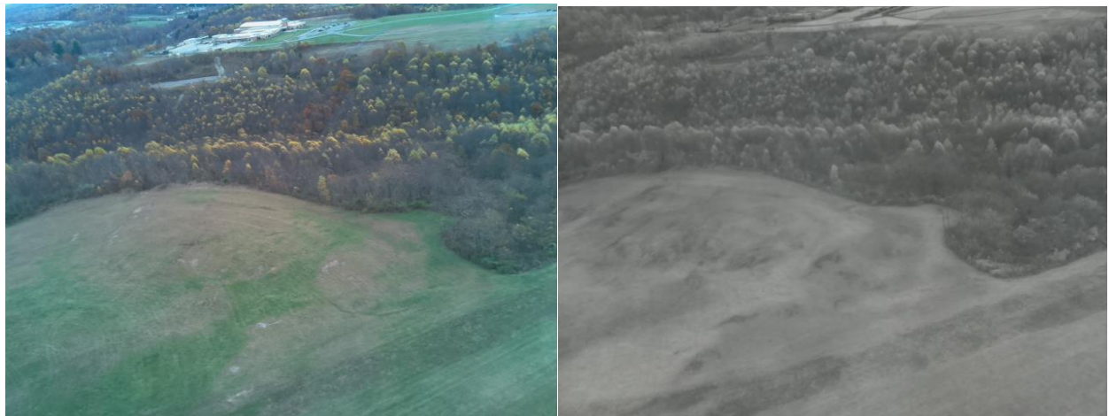
Figure 61: Original RGB (left) and NIR (right) Images of Woodline and Field Taken with General Aviation Aircraft at 250 ft AGL
