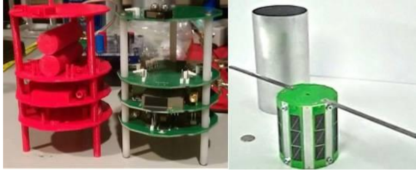
Figure 26: 3D Printed Model Next to Stacked Assembly of IOS TubeSat Kit (left) and a Fully Assembled Tubesat (right)
