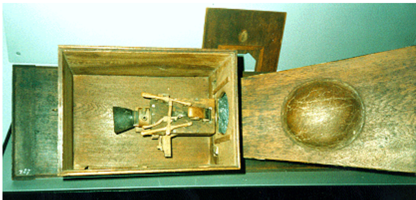
Figure 3-1: Wolfgang Von Kempelen's Talking Machine [33]
