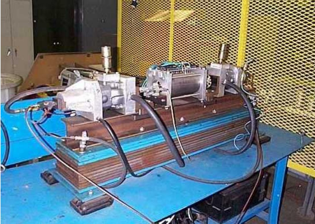
Figure 2.10. Experimental Prototype of Two-Stroke Compression-Ignition Linear Engine
