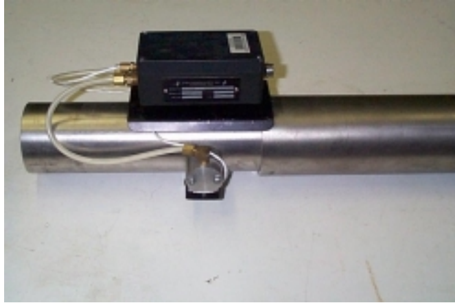
Figure 10 J-TEC VE503 Exhaust Vortex Shedder on original tube
