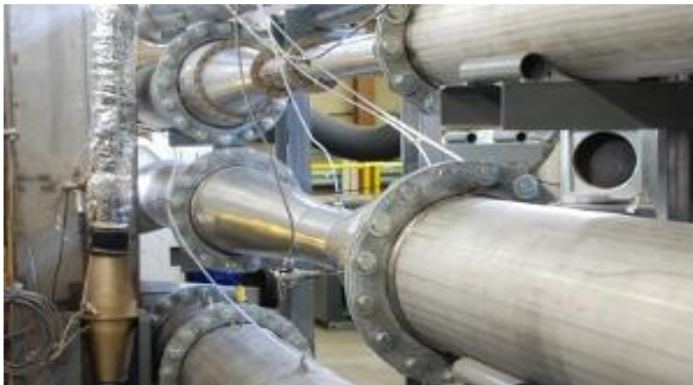
Figure 5: Full scale dilution tunnel constant volume sampling system
