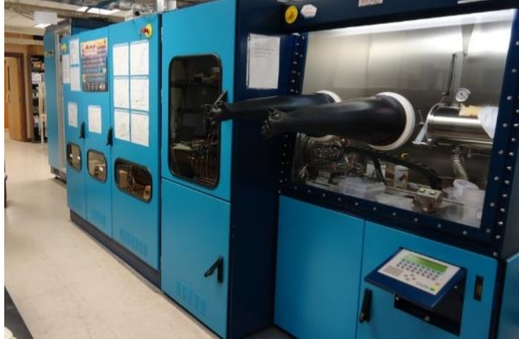
Figure 2.5: Picture of the Aixtron 200/RF-S MOVPE system used for the growth of all III-nitride materials used in this work.
