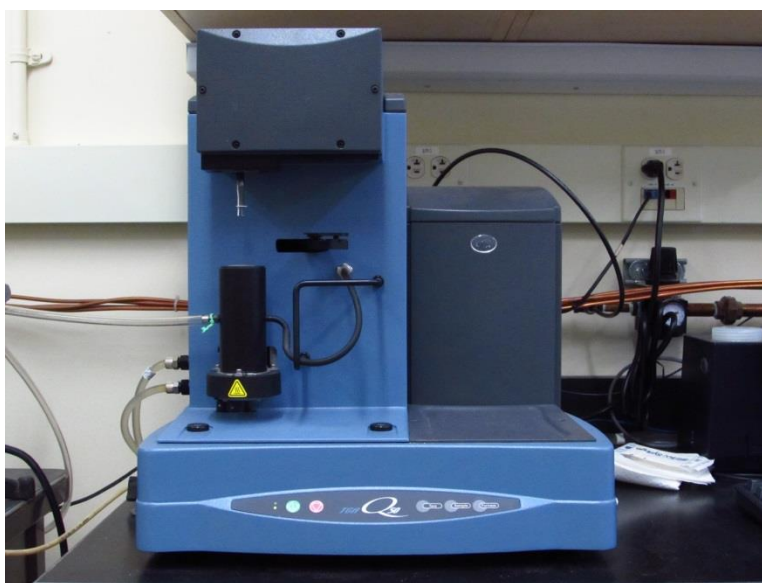
Fig. 3.2 A photograph of the commercial Q50 TGA system used for experiments.
