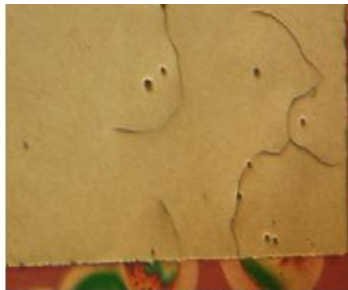
Figure 5.18: Optical images of the AlN air-bridge after re-sputtering platinum contacts on the bridges
