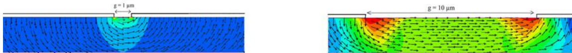
Figure 5.8: Electric field generated in a piezoelectric film with electrode gaps (a) 1 \mu\text{m} (b) 10 \mu\text{m} . Modified from [104].
