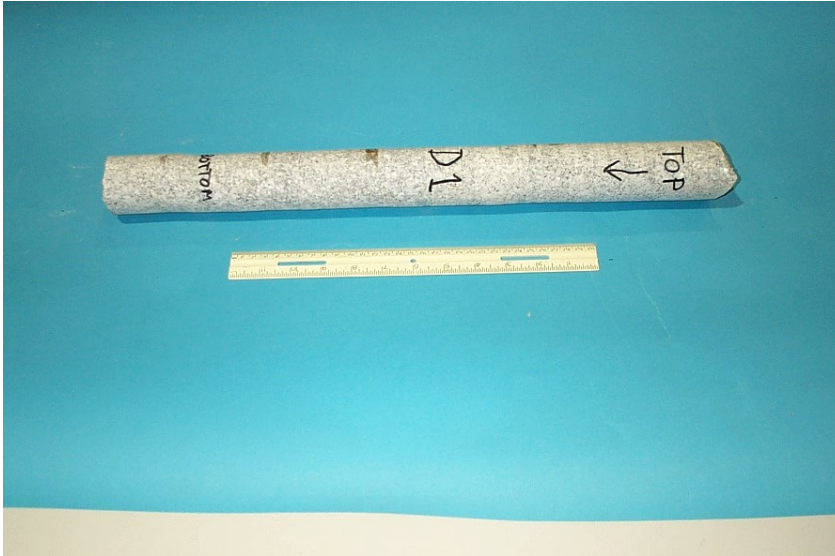
Figure 4.16 Sample of Core Collected from Barre Granite Rock Media
