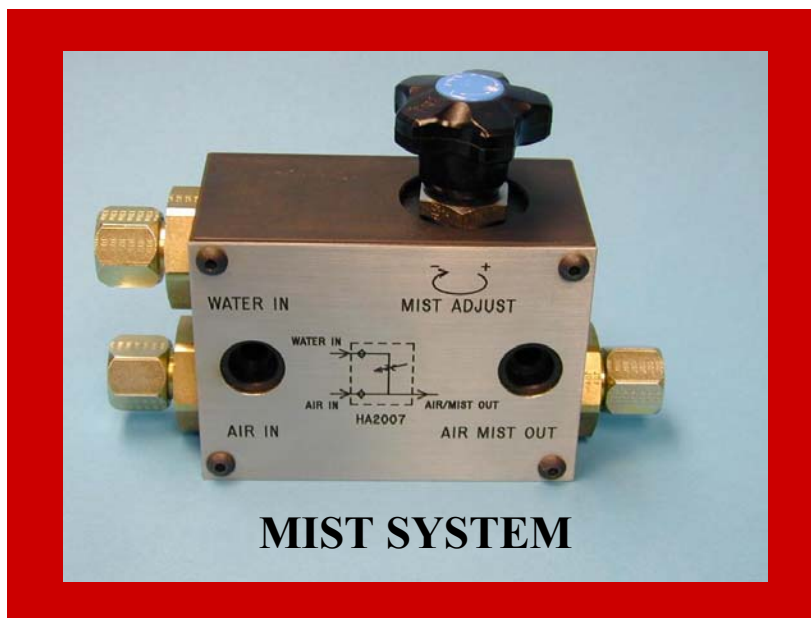
Figure 4.19 Photograph of “Mist” System Used During Noise Testing
