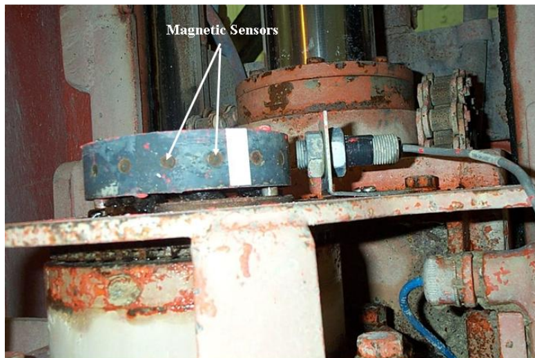
Figure 4.12 Pulser Disk and Electro-sensors Mounted on Drill Chuck
