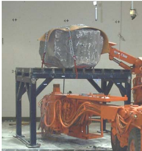
Figure 4.3 Test Fixture in Reverberation Room.
