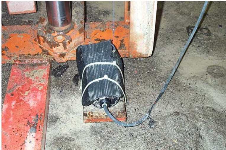
Figure 4.13 Location of String Potentiometer for Determination of Penetration Rate
