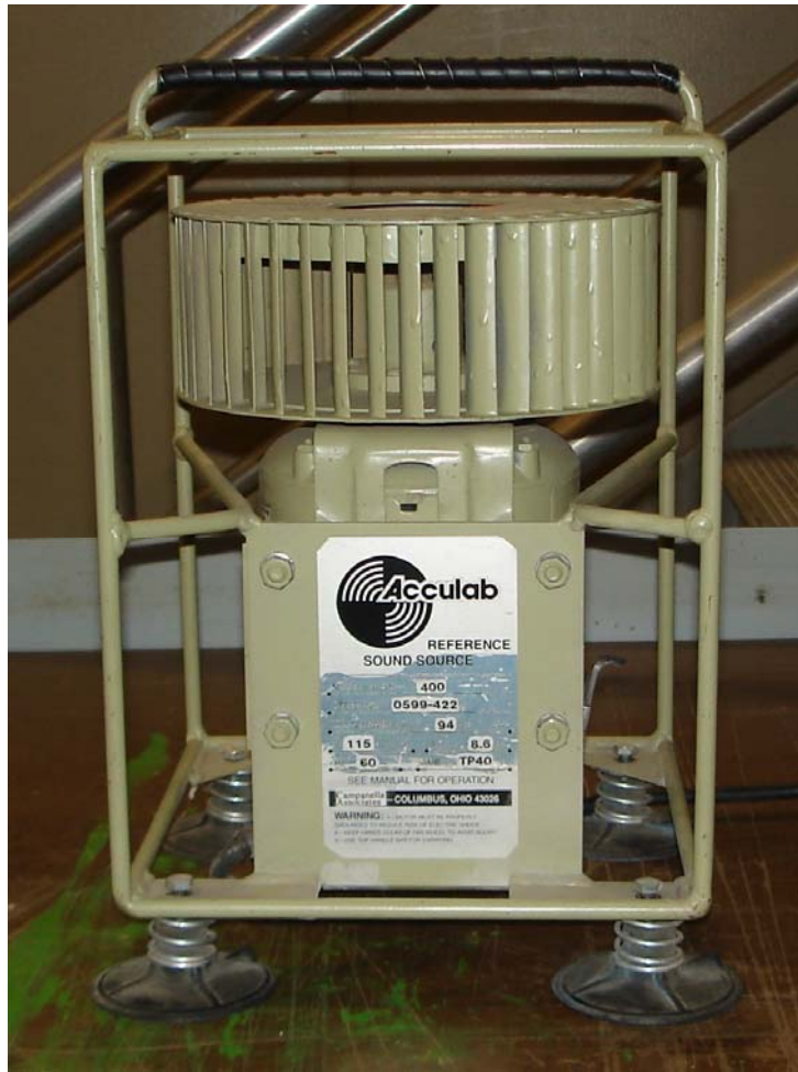
Figure 6.10 Photograph of Calibrated Sound Source for Underground Testing
