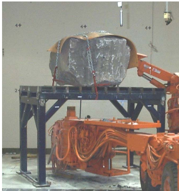
Figure 1.3 Noise Testing of Roof Bolter in Reverberation Room
