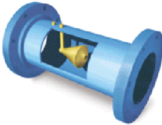
Figure 3.8 A cutout of the V-Cone showing the conical mass in the center of the flow, and the pressure ports.
