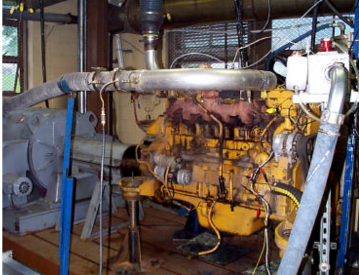
Figure 3.1 The WVU EERL test cell with an engine on the dynamometer, and the exhaust system. The Annubar ® can be seen in the upper left hand corner.
