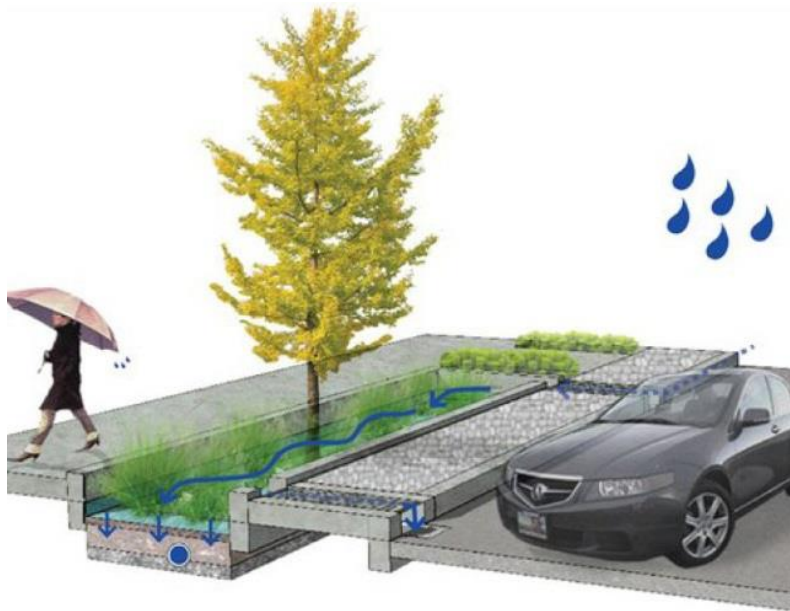
Figure 28. Bioretention System on Street
