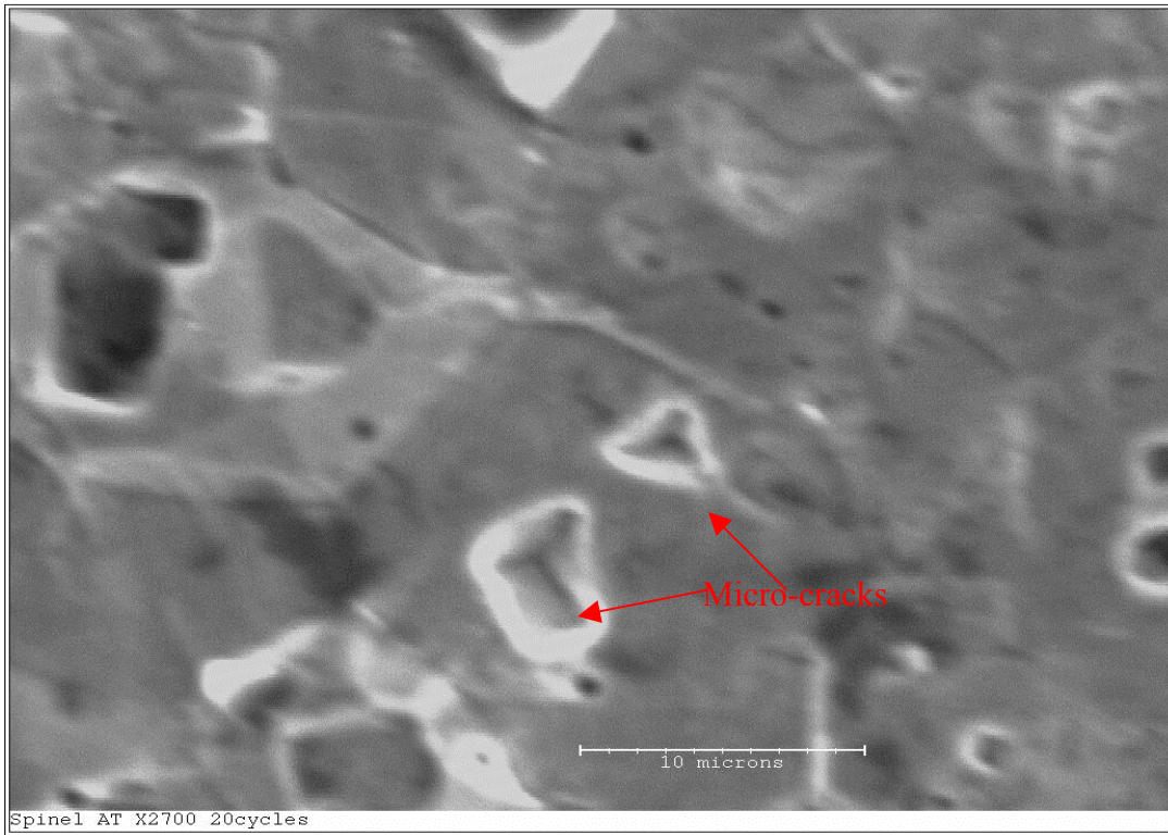
Figure 4.45 Clear view of the triangular cracks in the molybdenum matrix at a magnification of 2700
