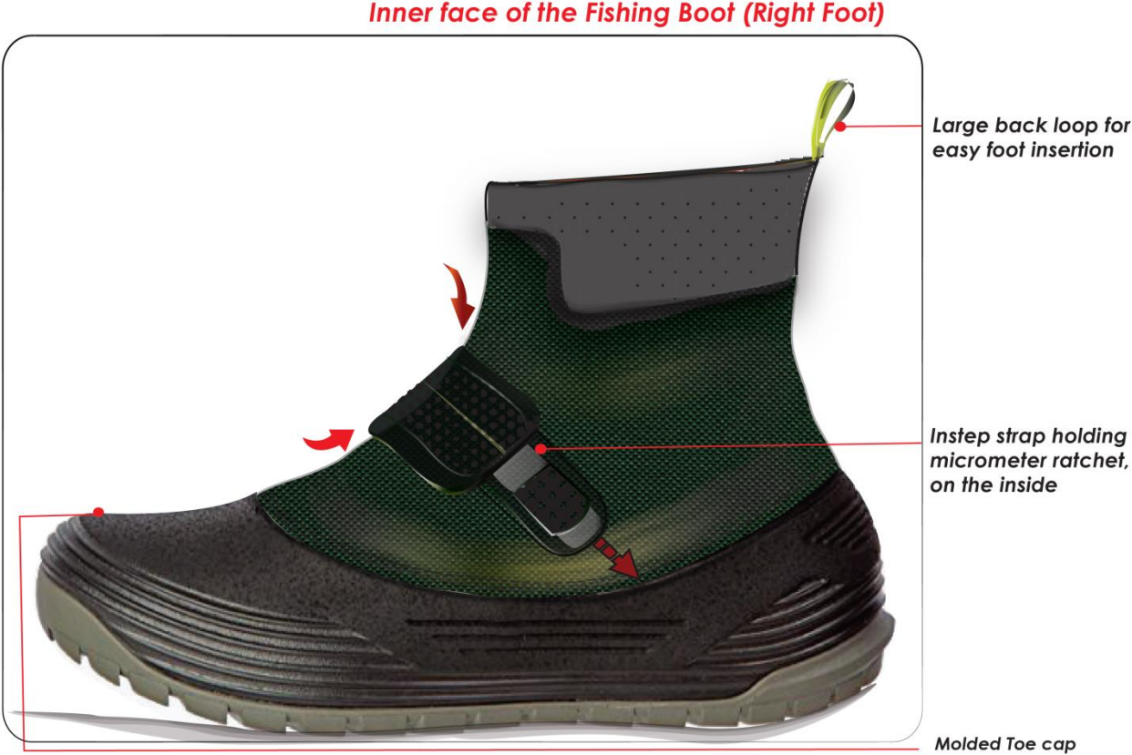
Figure 39: Detailed Design - Inner Face (right foot)
