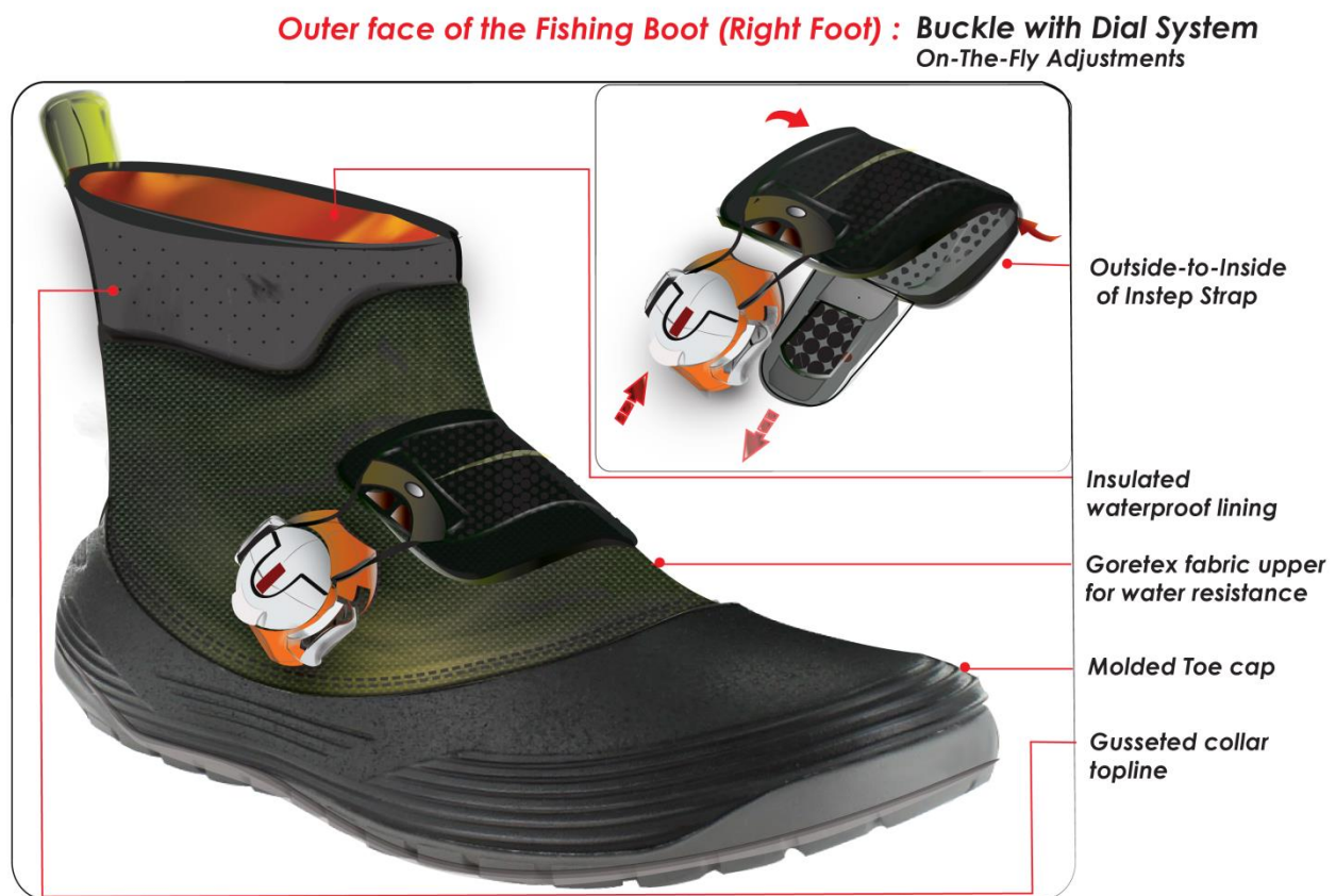
Figure 38: Detailed Design - Full View of the Boot (right foot)
