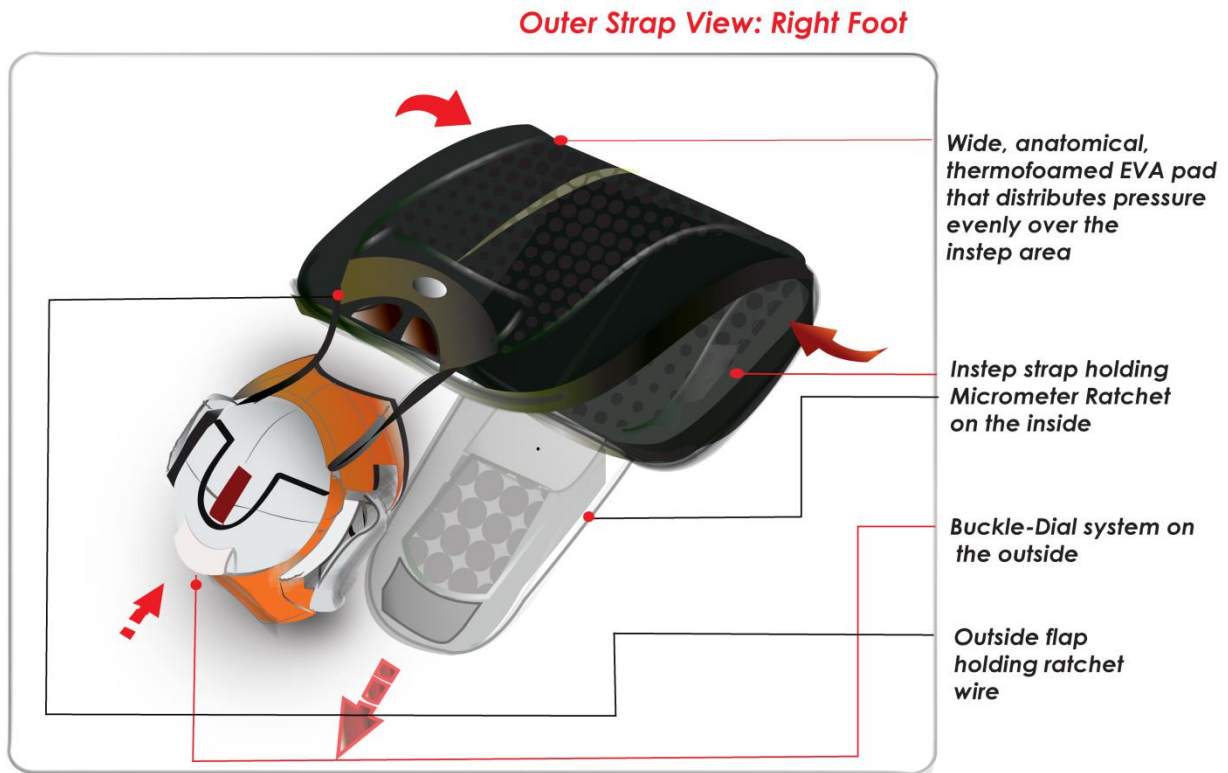
Figure 40: Detailed Design - Outer Strap
