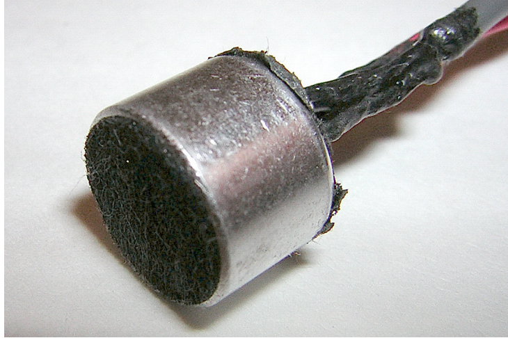
Figure 40: The fast response microphone used in the shock tube experiments.
