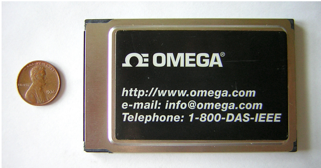
Figure 42: The Omega DAQP-208H PCMCIA card was used to collect experimental data.
