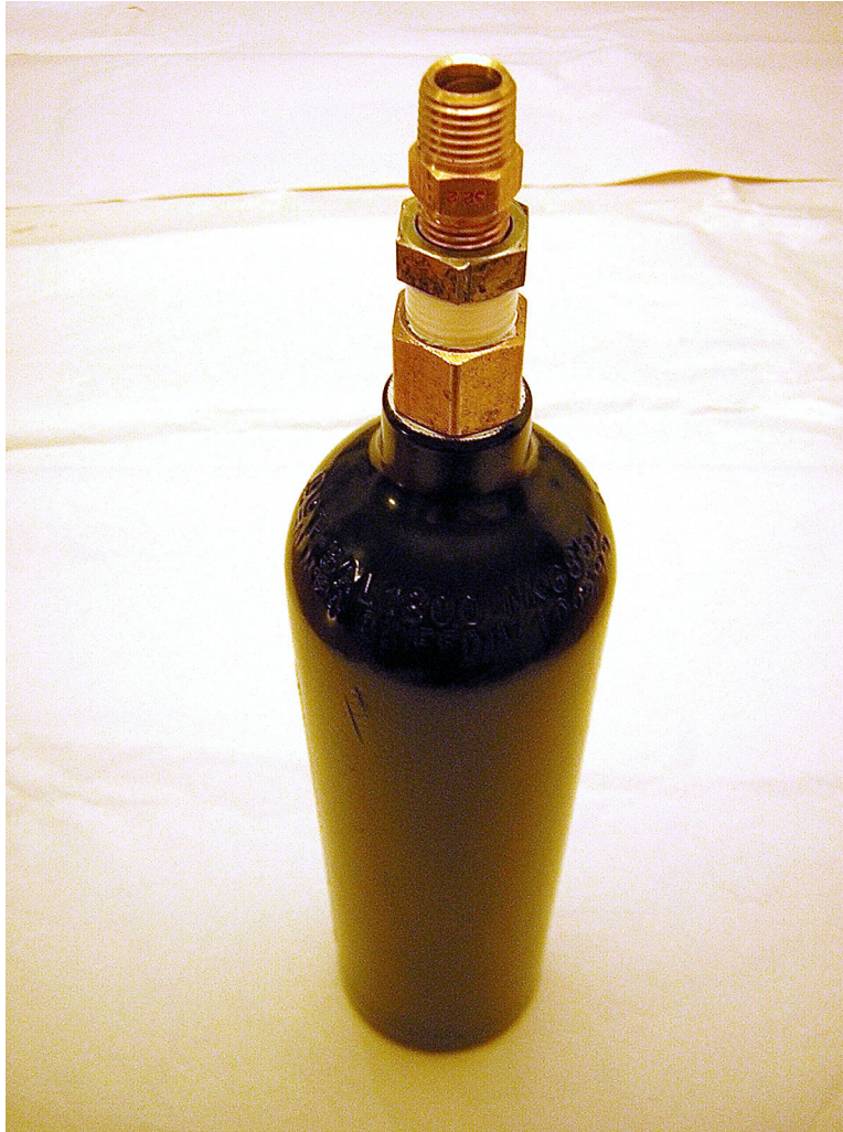
Figure 38: A modified CO 2 bottle was used as the downstream constant volume (543cc) tank in many of the constant volume tests.
