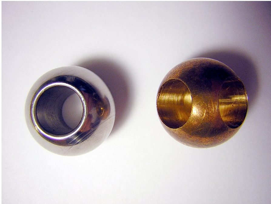
Figure 27: The original ball (left) which had a straight 0.371” hole was replaced with a new ball (right) which had a 90° 0.375” hole.
