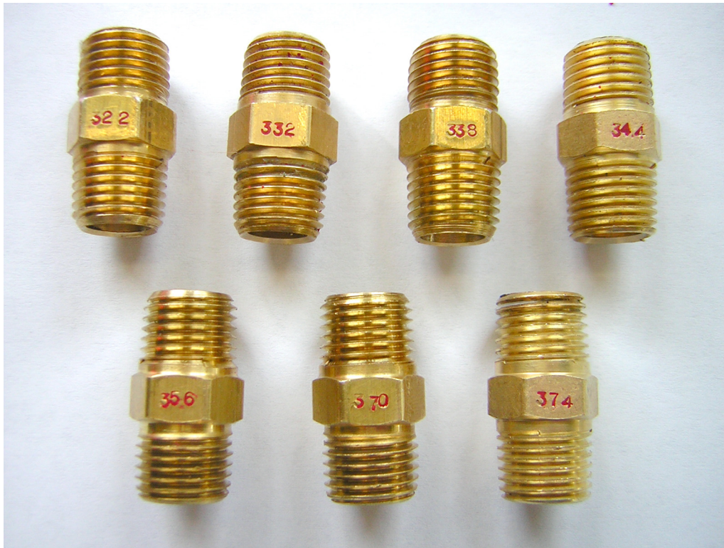
Figure 29: Nozzles of various diameters were used to force the flow to choke at the exit of the CCV (diameters in thousandths of an inch are stamped on the nozzle bodies).
