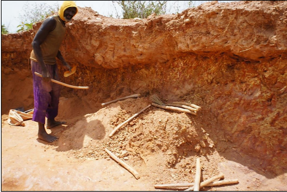
Figure 3. ASM activity targeting the gravel layer below the lateritic upper crust. Photo credit: Peter Chirico, USGS, February 2013.
