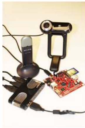
Figure 3.1: Smart camera unit: Assembled using a Beagleboard, Logitech 9000 camera and a 802.11 wireless card
