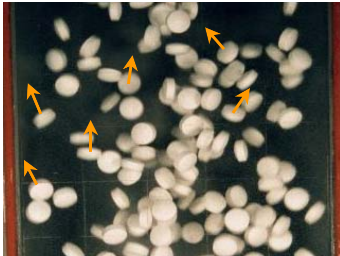
Figure 4.8: Image of tablets in fluidized bed - spouted region, (Subramanian, 2000), arrows show possible directions of particle movement.
