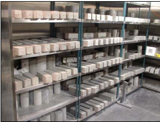
Fig 5.2 - Storage of shrinkage specimens
