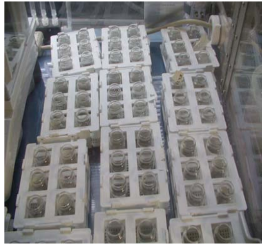
Fig 4.5 - D-dried samples kept within the RH chamber for water adsorption
