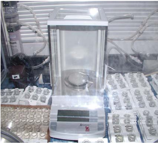
Fig 4.4 - A four place of decimal balance used for weight measurement placed within the RH chamber
