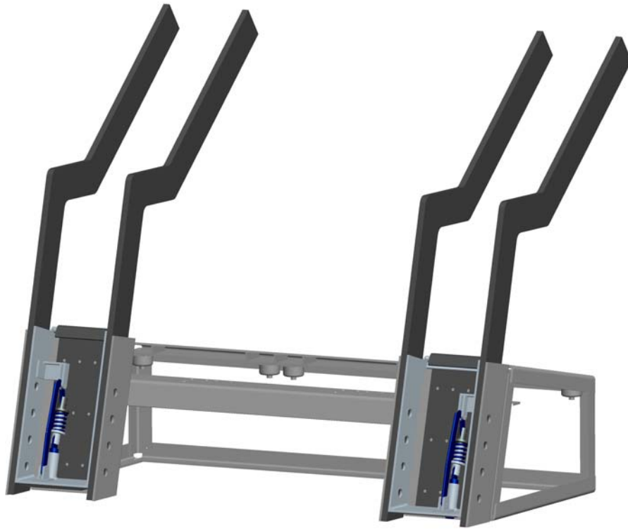
Figure 14: Pod and Arms with Quick Attach Locked
