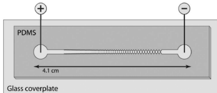
Figure 2-6. Schematic of the direct current insulator gradient dielectrophoresis device. An insulated sawtooth pattern is integrated with a tapered microfluidic channel to generate localized non-uniform electric field gradients of increasing strength from left to right.
