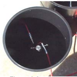
Figure 3.2a Specimen Mold with strain gauge top view
