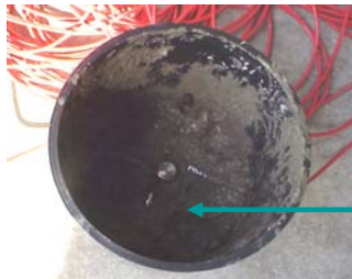
Figure 3.2e Specimen Mold with strain gauge top view partially filled with concrete
