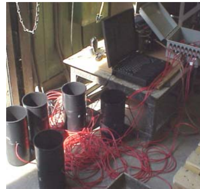
Figure 3.2c Instrumented Molds connected to multiplexer
