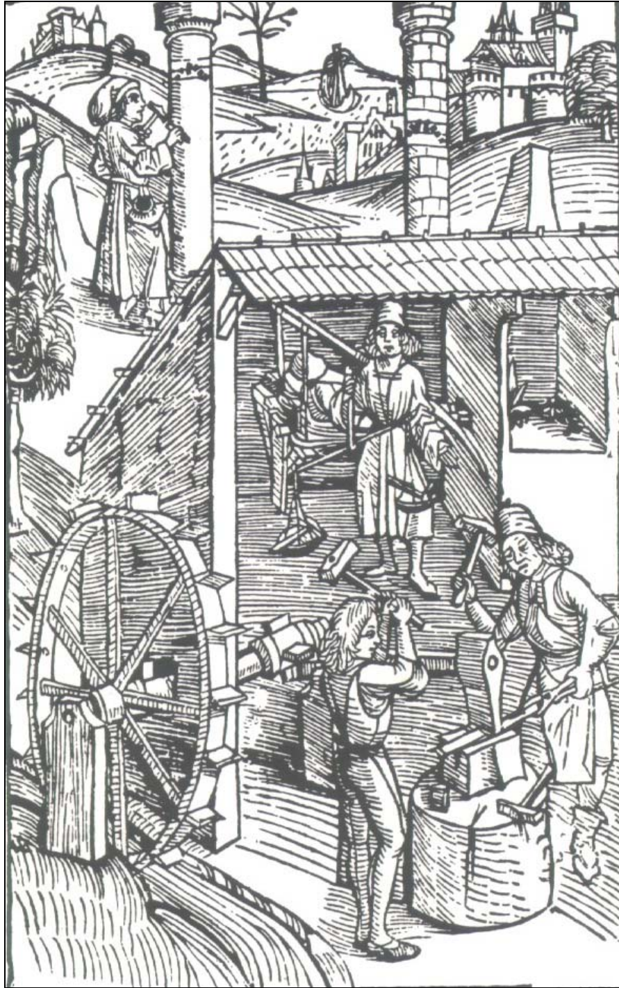
Figure 2-1: Trip hammer in a smithy, an example of the extension of the water wheel's utility by the conversion of continuous rotation into periodic "up-and-down" motion. (From Spechtshart's "Flores musicae").
