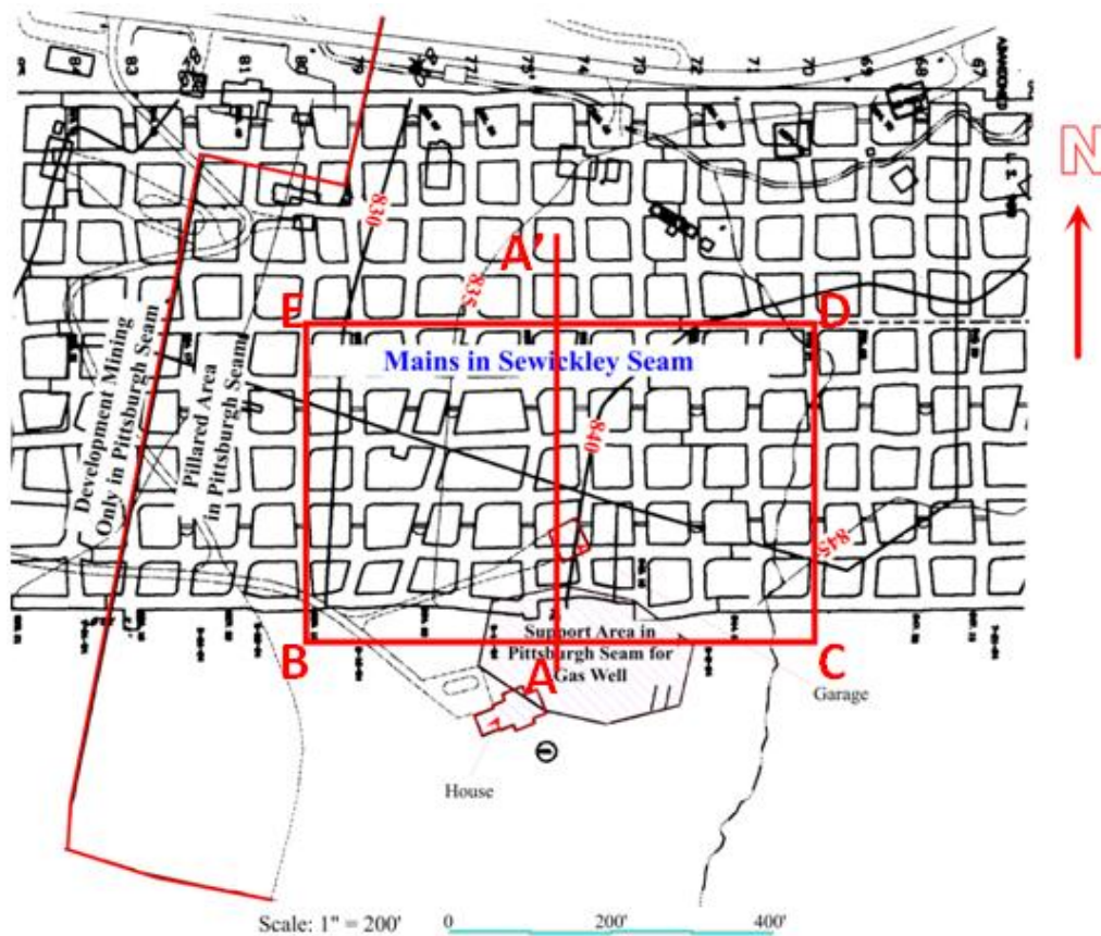
Figure 5.9 Spatial relationships among surface structures and mains in the mines in the Sewickley and Pittsburgh Seams
