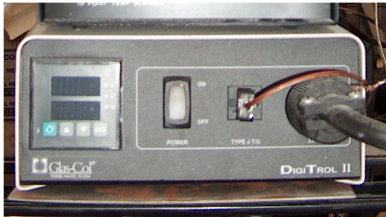
Figure 14 WFE Temperature controller
