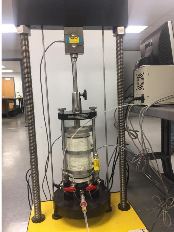
*Figure 4. Display of the ICU triaxial test*
