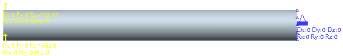
Figure 17 – Static loads applied to shaft root diameter
