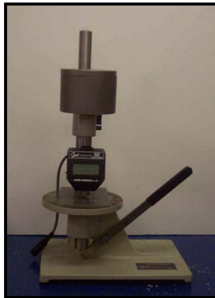
Figure 5-28 Durometer hardness used to measure the hardness of polycarbonate
