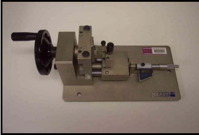
Figure 2-7 Notcher used to notches according to the ASTM standard
