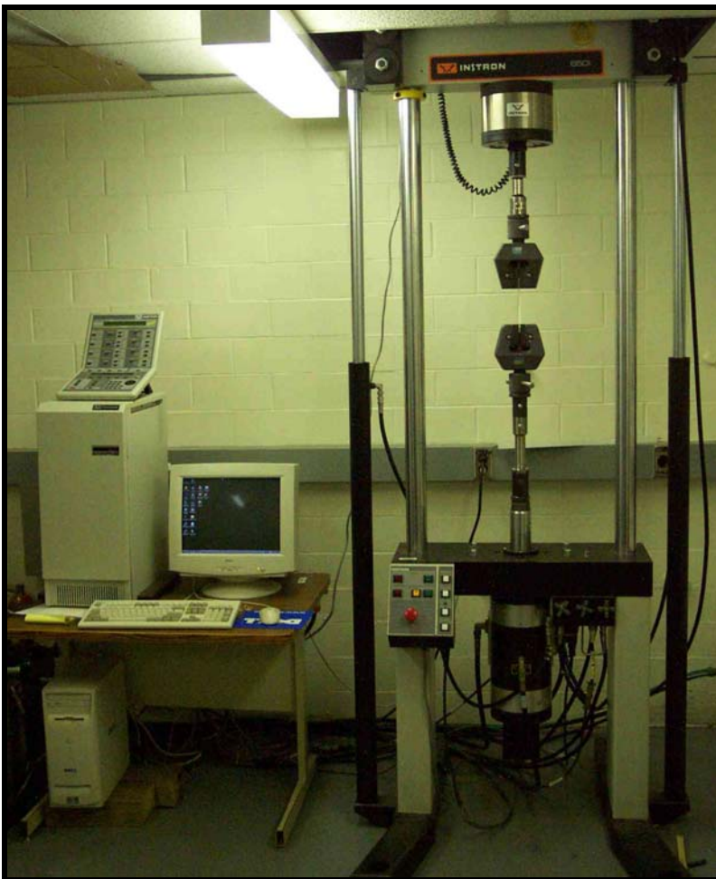
Figure 5-4 Instron machine used to measure the tensile and flexural strength
