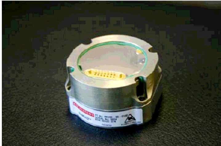
Figure 2.3: SiIMU02 IMU Developed by BAE Systems for ERGM Research
